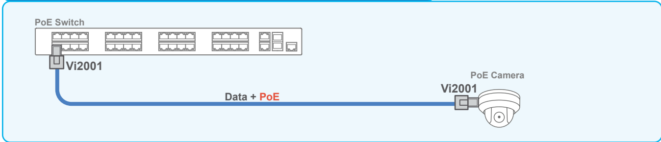
The Vi2001 can protect networking equipment against damaging voltage surges over standard distance UTP cables.
