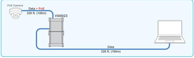
The Vi00023 enables connecting to a laptop using a wired connection.
