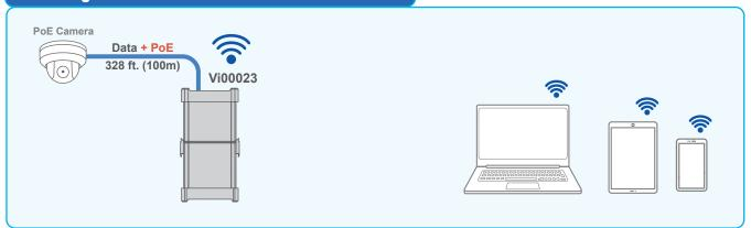
The Vi00023 enables connecting the PoE cameras to any wireless device using a WiFi connection.
