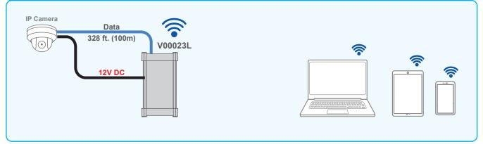
The Vi00023L enables connecting the non PoE cameras to any wireless device using a WiFi connection.
