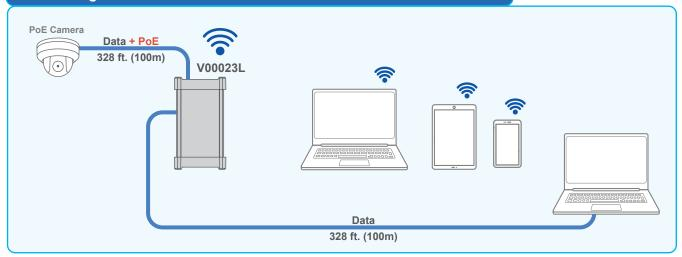
The Vi00023L has a built in switch that makes it possible to connect an IP camera to a network of wired and wireless devices.
