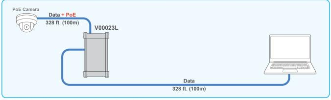
The Vi00023L enables connecting to a laptop using a wired connection.
