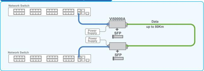
With 1000Mbps (1G) bandwidth, the Vi50000A is the perfect solution for connecting network switches over long distances.
