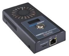
Vigitron's patent pending Vi00024 is an innovative test tool that installation reliability by measuring PoE capacity at any point of a networks before installing a camera. The Vi00024 simulates PoE devices and measures the maximum PoE capacity received from the PoE source over the network. It is compliant with IEEE 802.3af/at/bt standard up to 74W.
