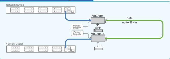
With 1000Mbps (1G) bandwidth, the Vi50000A can be used with the Vi50001 as a perfect solution for connecting network switches over long distances.
