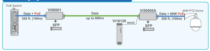
The Vi50000A is used with the Vi50001 for long distance high bandwidth applications. The Vi50000A provides up to 60W PoE power to meet the highest PTZ dome power requirements.
