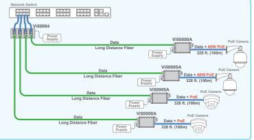
The Vi50004 along with Vi50000A enables addging 100/1000 Base-T fiber connection to any network switch. Each port of Vi50004 can be individually powered by PoE or local power supply SFPs need to be added to Vi50004 and Vi50000A to match the fiber optic cable
