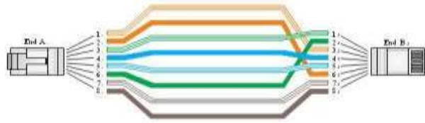
Figure 21: Crossover Wiring
