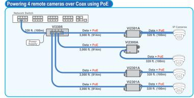
Up to four cameras, including high powered PTZ domes can be remotely powered without the need for local power supplies.
