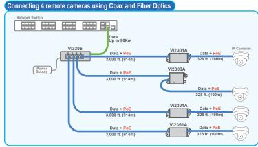
The Fiber optics uplink port can be used to connect 4 cameras up to 80Km.
