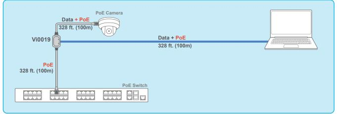
The Vi0019 enables connecting to a laptop using a wired connection to setup and focus cameras.
