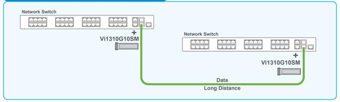
The Vi1310G10SM can connect 2 network switches at long distances at 10,000Mbps data rate.
