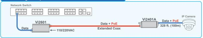
The Vi2601 and Vi2401A provide a reliable power source for the long distance and higher power requirements of PTZ domes and IP cameras with power surges due to accessory features such as day/night, LED operations, and auto focus with heater/blower functions.
