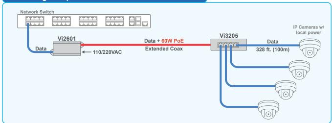
The Vi2601 and Vi3205 eliminate the need for any local network switch power, while providing a single coax path for transmitting four cameras from remote locations. This combination simplifies installation and reduces costs.
