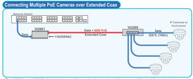
The Vi2601 and Vi3205 eliminate the need for any local network switch power, while providing a single coax path for transmitting four cameras from remote locations. This combination simplifies installation and reduces costs.
