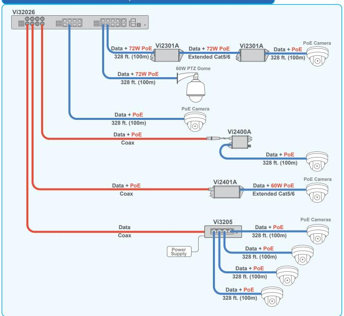
The Vi32026 can transmit data and PoE up to 36W over Coax and up to 72W over standard UTP cables.
