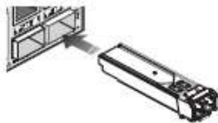
Figure 12: Inserting an SFP Transceiver into a Slot
