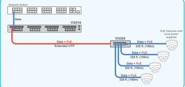
The Vi3205 can receive data and PoE power for powering itself over extended distance Coax up to 3,000 ft. at 100Mbps. The cameras use local power supplies.
