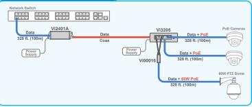
The Vi3205 can receive data over extended distance Coax up to 3,000 ft. at 100Mbps and power 60W PoE cameras using the Vi00016 combiner cable and a local power supply.
