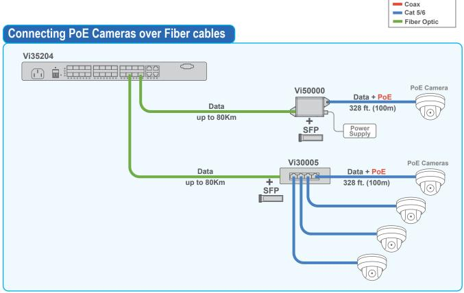
Vigitron media converters and switches with Fiber connection can be used with Vi35024 to provide PoE to cameras or other PoE devices.
