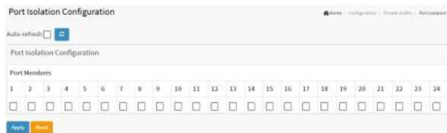
Figure 2.16.2: The Port Isolation Configuration
