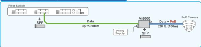
By using the SFPs, the Vi5001 will be compatible with most installed fiber types and can be directly connected to SFP modules installed in network switches.
