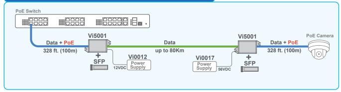
The Vi5001s are used for long distance high bandwidth transmission applications. The Vi5001 provides up to 30W PoE power to meet the high power requirements. of PoE cameras.
