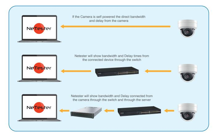
NeTester can be used at any point in the network to determine transmission performance.
