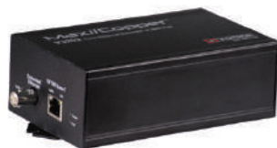
Vi3202 Single Port Coax PoE Midspan Power Input: 24VAC/DC PoE Output: 802.3af/af/bt (60W) Distance: up to 5000feet (1524m) Data: 10/100Mbps
