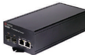
Vi3004LV 4-Port L2 PoE Switch 2 Copper Ports, 2 Fiber Ports Power Input: 24VDC PoE Output: 802.3af/at/bt (60W) Data: 10/100/1000Mbps
