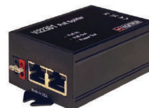
Vi22301 Single Port PoE Splitter PoE input: 802.3af/at/bt (60W) PoE Output: 802.3af/at (30W) Power Output: 12/24VDC (30W) Data: 10/100Mbps
