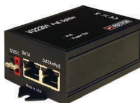
Vi22201 Single Port PoE Splitter PoE input: 802.3af/at (30W) Power Output: 12/24VDC Data: 10/100Mbps
