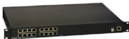
Vi2508 8-Port Extended UTP PoE Midspan PoE Output: 802.3af/at/bt (74W) Distance: up to 3000feet (909m) Data: 10/100Mbps
