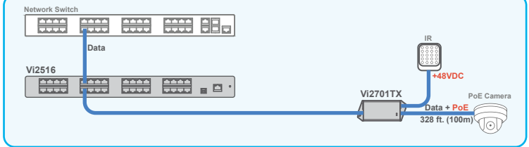
The Vi2701TX can be used with a Vi2516 extended UTP PoE Midspan to power a PoE camera and provide DC power to an IR light.
