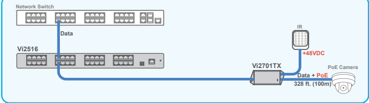
The Vi2701TX can be used with a Vi2516 extended UTP PoE Midspan to power a PoE camera and provide DC power to an IR light.
