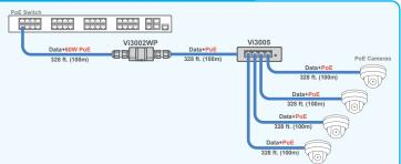
The Vi3002 can be used to connect multiple PoE cameras at extended distances
