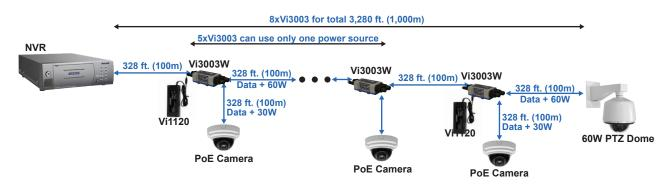
A total of 9 IP addresses can be accessed on a single cable run, eliminating the need for network switches.
