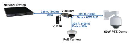
Vi3003W allows for the transmission of two cameras over a single camera run or adding a new camera close to an existing camera.
