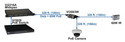
Vi3003W allows for the transmission of data for a camera and an IR illuminator over a single camera run. The PoE Midspan provides power to the Vi3003W ,camera and IR illuminator.
