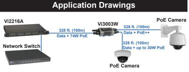
Vi3003W allows for the transmission of two cameras over a single camera run or adding a new camera close to an existing camera.
