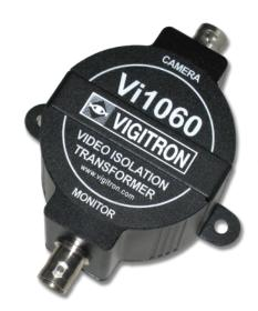
The Vigitron Vi1060 is a high resolution video isolation transformer designed for base-band composite video signals. The annoying and potentially damaging hum bars on the screen are caused by ground voltage potential differences between your video equipment that is called ground loop. The Vi1060 provides complete isolation between devices and eliminates video hum bars, ground loops, and DC offsets which can degrade picture quality and potentially damage video equipment.
