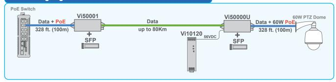
The Vi50000U is used with the Vi50001 for long distance high bandwidth applications. The Vi50000U provides up to 65W PoE power to meet the highest PTZ dome power requirements.
