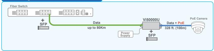
By using the SFPs, the Vi50000U will be compatible with most installed fiber types and can be directly connected to SFP modules installed in network switches.
