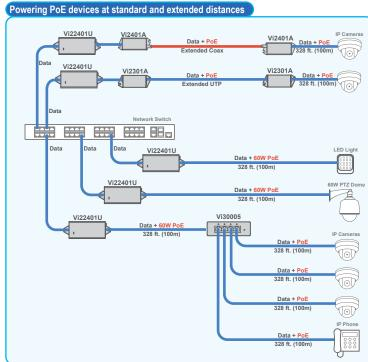
The Vi22401 can power a wide range of PoE devices at standard and extended distances up to 60W.
