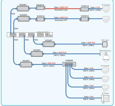
The Vi22401 can power a wide range of PoE devices at standard and extended distances up to 60W.
