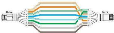
Figure 21: Crossover Wiring 1000Base-T Pin Assignments
