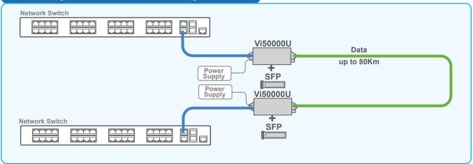
With 1000Mbps (1G) bandwidth, the Vi50000U is the perfect solution for connecting network switches over long distances.
