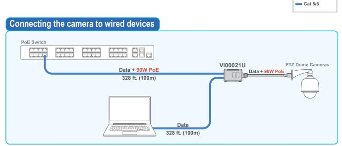
The Vi00021U enables connecting to a laptop using a wired connection to setup and focus IP cameras.
