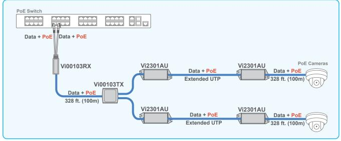
The NetMux<sup>™</sup> Vi00103 along with Vi2300 series can connect two cameras at extended UTP distances.
