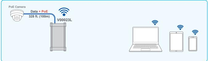
The Vi00023L enables connecting the PoE cameras to any wireless device using a WiFi connection.
