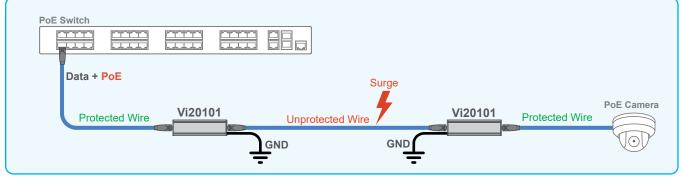
The Vi20101 can protect networking source equipment and Cameras against damaging voltage surges.
