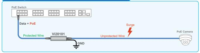
The Vi20101 can protect networking source equipment against damaging voltage surges.
