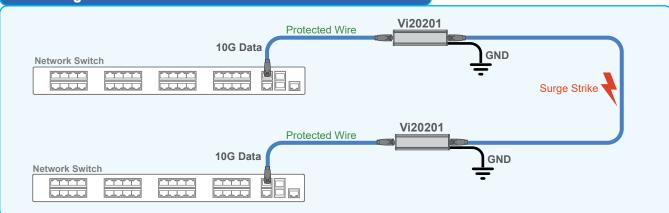
The Vi20201 can protect networking equipment close to it against damaging voltage surges.
