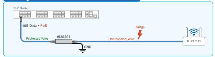
The Vi20201 can protect networking source equipment against damaging voltage surges.
