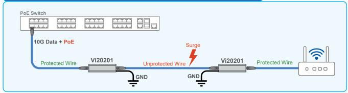
The Vi20201 can protect networking source equipment and remote devices against damaging voltage surges.
